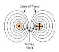
The strength of the magnetic field on the magnitude of the electric current. The higher the current, the stronger the magnetic field, and therefore the greater the deflection. The strength of the magnetic field decreases as you move further from the conductor. There will be less deflection as the compass is drawn from the current-carrying conductor.
