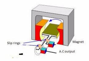
When the coil is vertical, no cutting of the magnetic lines of force takes place although the number of lines linking the coil is maximum. The rate of change magnetic flux is zero and as a result, no a.m. is induced in the coil.
