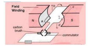
When the loop is rotated in the magnetic field, the induced e.m.f is still in alternating form. However after rotation of  $180^{\circ}$  instead of the current reversing, the connections to the external circuit are reversed so that the current direction in the external circuit remains the same.
